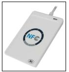
The ACR122U is a PC-linked contactless smart card reader/writer developed on the 13.56 MHz contactless technology. It is the world's first CCID-compliant contactless card reader/writer that follows both ISO 14443 and ISO 18092. This device is designed to support not only Mifare and ISO 14443 Type A and B cards, but also FeliCa and NFC tags.
